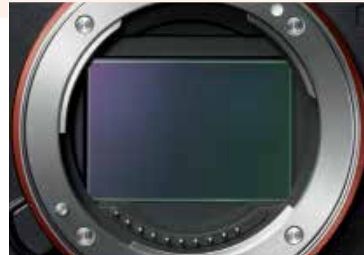
Left: The state-of-the-art, 42-megapixel full-frame (36 x 24mm) sensor at the heart of the Sony Alpha 7rii.
